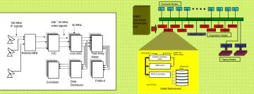
**PuMa-II hardware** is composed of a 42-node Linux Cluster. The cluster is logically separated into acquisition and compute nodes. See diagram above. Each node consists of dual Opertron processors clocked at 2GHz, a high performance mother board and 2GBytes of physical RAM. The complete instrument features ~400 GFlops of computational power, ~50 TeraBytes of storage space and can sustain a data throughput of 640 Mbytes/sec for 12 hours.
