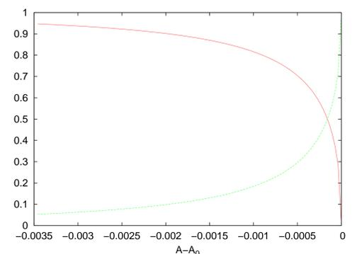
Figure 3: Reflection (green) and transmission (red) coefficients for the o-mode incident upon a shear in bulk plasma velocity. The region of the incident wave has  $\gamma = 600$  which bounds plasma with  $\gamma = 800$ .  $r = 100R$  and  $\eta = 10^{-3}$ . The eigenvalues are imaginary in both regions.  $A_0$  is the degeneracy point.
