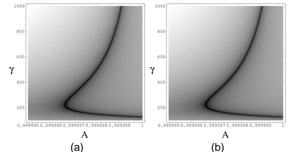
Figure 2: Grey-scale plots of the Log of the absolute value of  $\gamma^3(1 - A\beta)^2 - X$ . The black region denotes where this term  $\rightarrow 0$  and thus where the o-mode is strongly reflected. To the left of this the eigenvalues are pure imaginary and to the right they are real.  $r = 10R$  and  $\eta = 1$  in (a), and  $r = 100R$  and  $\eta = 10^{-3}$  in (b).
