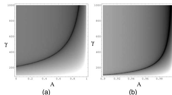
Figure 1: Grey-scale plots of the Log of the absolute value of the term in square brackets in (7). The black region denotes where this term  $\rightarrow 0$ , i.e. where strong coupling occurs. Above this the eigenvalues are complex (both real and imaginary parts) and below they are real or pure imaginary.  $r = 10R$  in (a) and  $r = 100R$  in (b).  $\eta = 10^{-3}$  in both.
