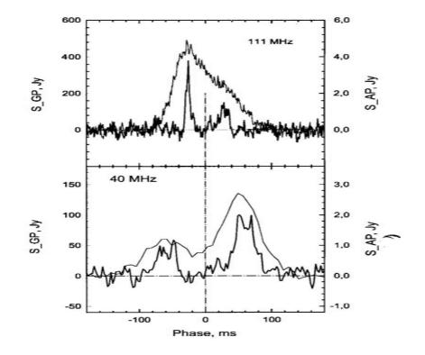
(top) The double GP of pulsar PSR B0031-07(bold line) observed at 111 MHz together with the AP (thin line),
