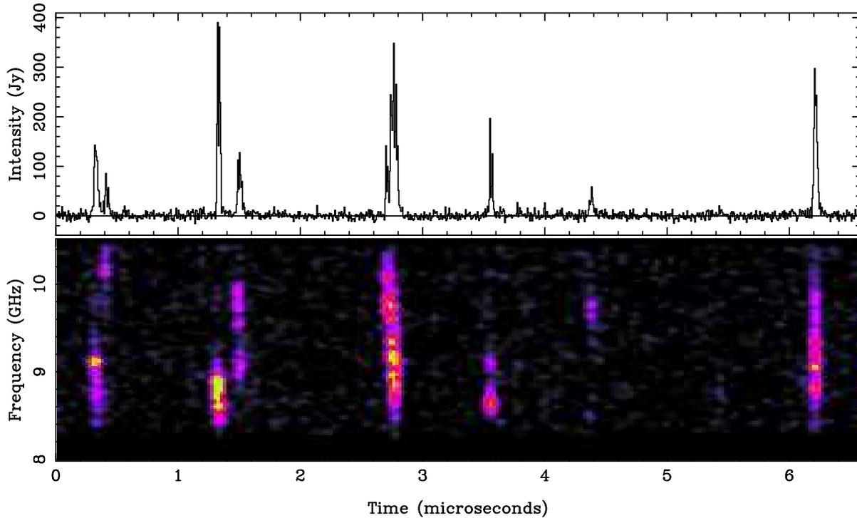
Blowing up the  $35.5 - 42\mu\text{s}$  region of the “sparse” MP shown in the previous figure. Some individual “shots” are apparent, and the relatively narrow-band spectrum ( $\delta\nu/\nu \sim 0.1$ ) of individual shots can be seen. Time resolution 6.4 ns; dynamic spectral resolution 19.5 MHz and 51 ns.
