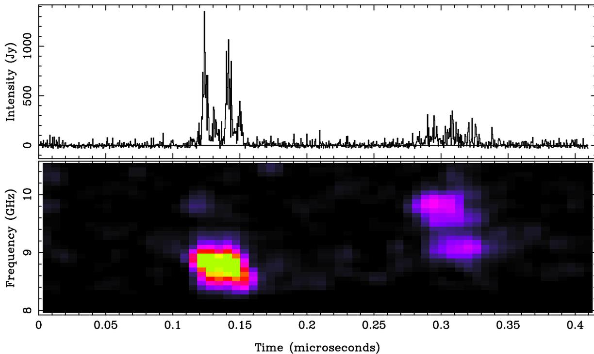
Blowing up the  $1.2 - 1.6\mu\text{s}$  region of the MP shown above, at our maximum time resolution, to reveal the temporal and spectral signature of individual nanoshots. Time resolution 0.4 ns; dynamic spectral resolution 78 MHz and 6.4 ns.
