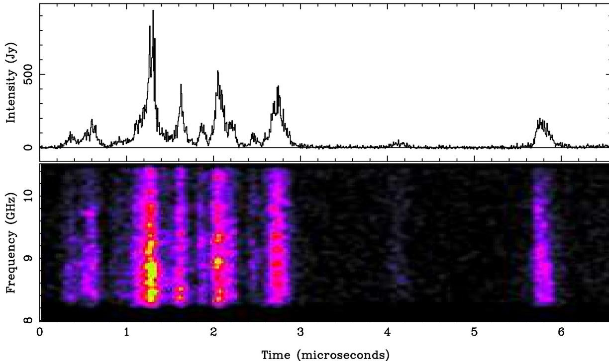
Most giant MPs consist of several **microbursts**, as shown here. The total intensity is plotted with time resolution 6.4 ns; the dynamic spectrum is plotted with 19.5 MHz spectral resolution and 51 ns time resolution. This and all data shown were observed at Arecibo and coherently dedispersed.
