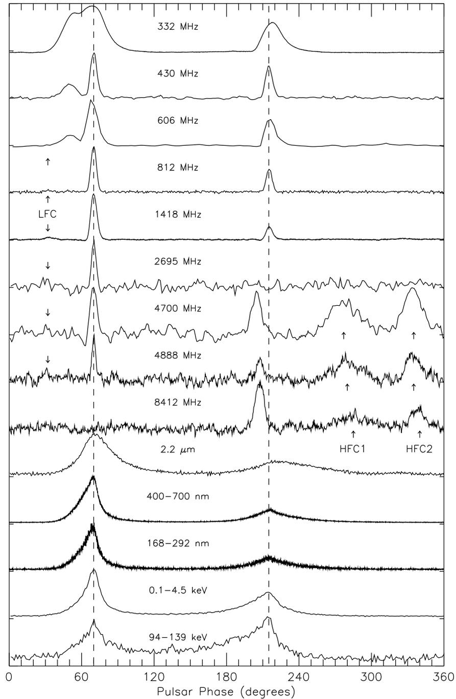
The mean profiles from the Crab pulsar show several frequency-dependent components. The **Main Pulse** and **Interpulse** are shown by the dashed lines at 70 and 215 degrees of rotation phase. They can be identified from low radio frequencies to hard X-rays. The Main Pulse becomes very weak and the Interpulse appears at a slightly different phase at high radio frequencies (Moffett Ph.D. thesis 1997).
