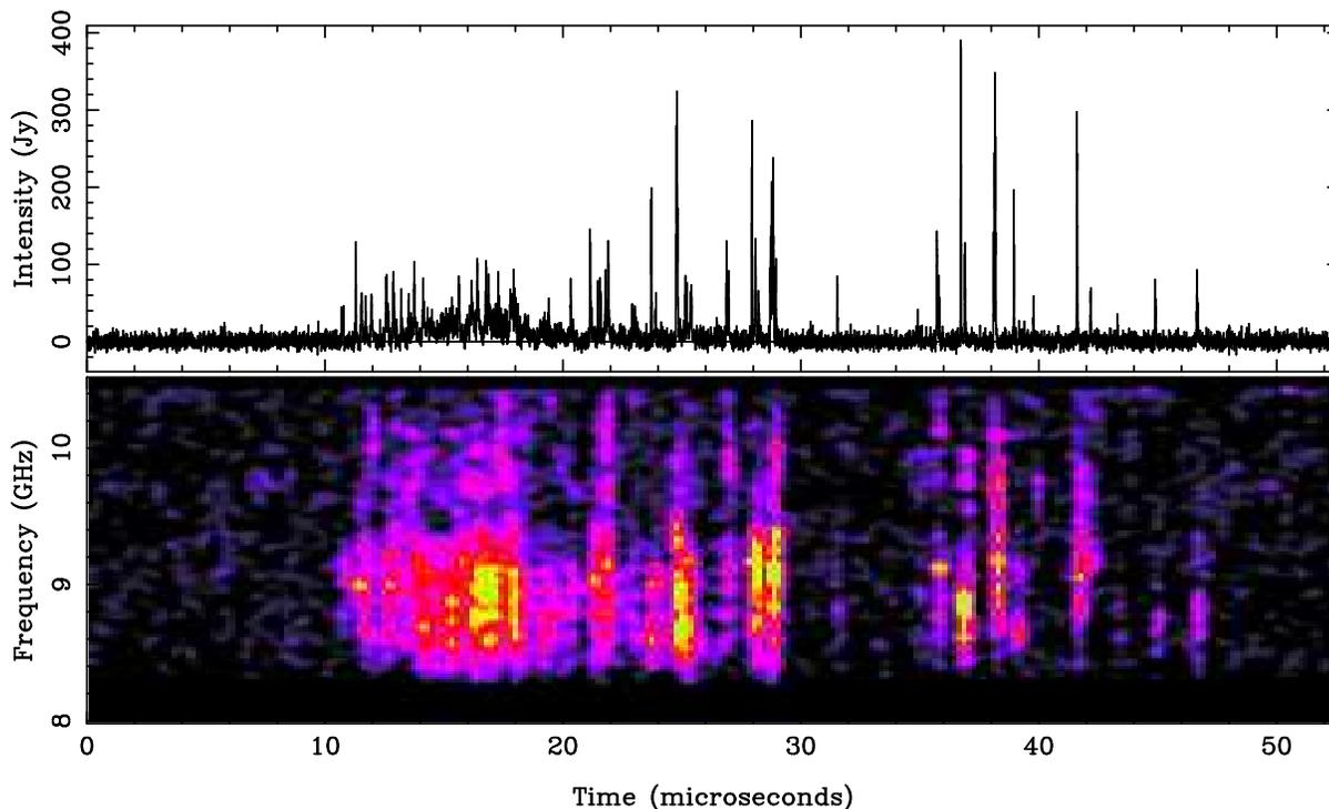
An occasional giant MP, however, consists of many short-lived **nanoshots**, which are well separated enough to be individually resolved. Time resolution 6.4 ns; dynamic spectral resolution 19.5 MHz and 406 ns. This pulse is shown at higher resolution in the next figures.
