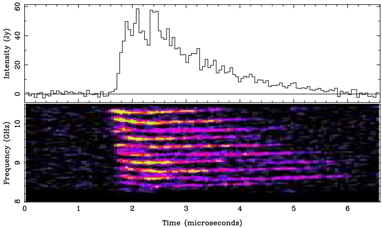
Two typical giant interulses. The dynamic spectrum of the interpulse contains several sets of **emission bands**, each of which lasts  $\sim$  a few  $\mu$ s. These bands appear in every giant IP, but not in giant MPs observed at the same time; thus they are neither instrumental nor interstellar. Time resolution 6.4 ns; dynamic spectral resolution 19.5 MHz and 52 ns.
